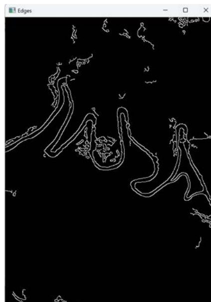
Fig. 3. The result obtained in binary format by applying the Canny algorithm
